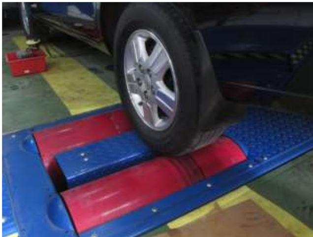
Gambar 2.2 Chasis dynamometer.
