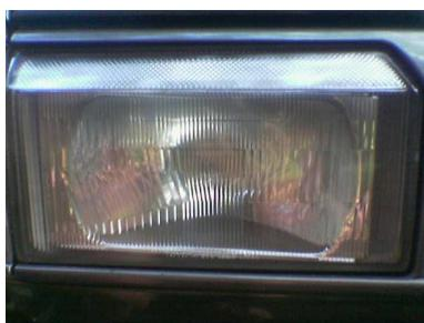
*Gambar 4. lampu tipe semi sealead beam*
