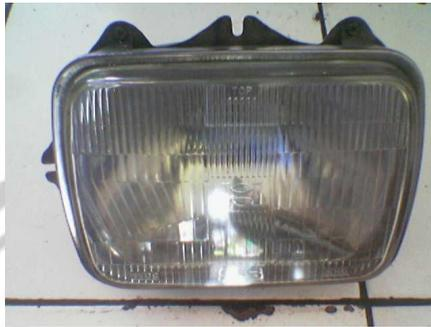
Gambar 3. lampu besar tipe *sealead beam*
