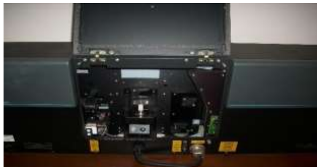
Gambar 3.8. Particle size- Analyzer (PSA) merk COULTER series LS100.
