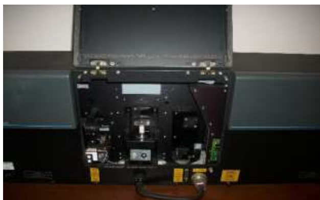
Gambar 3.9. Particle size- analyzer (PSA) merk Coulter series LS100.
