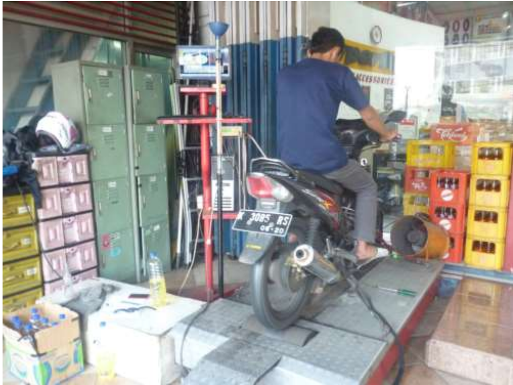
Gambar 3. Pengujian performa mesin di Dynotest Hyperspeed Semarang
