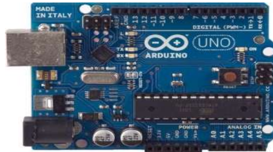
Gambar 2.13 Board Arduino Uno
