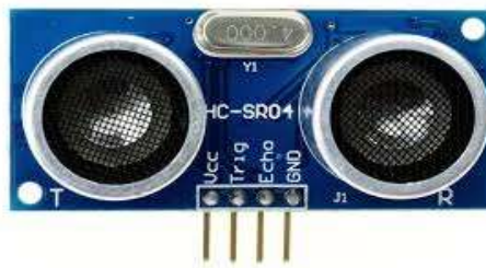
Gambar 2.10 Sensor Ultrasonik HC-SR04
