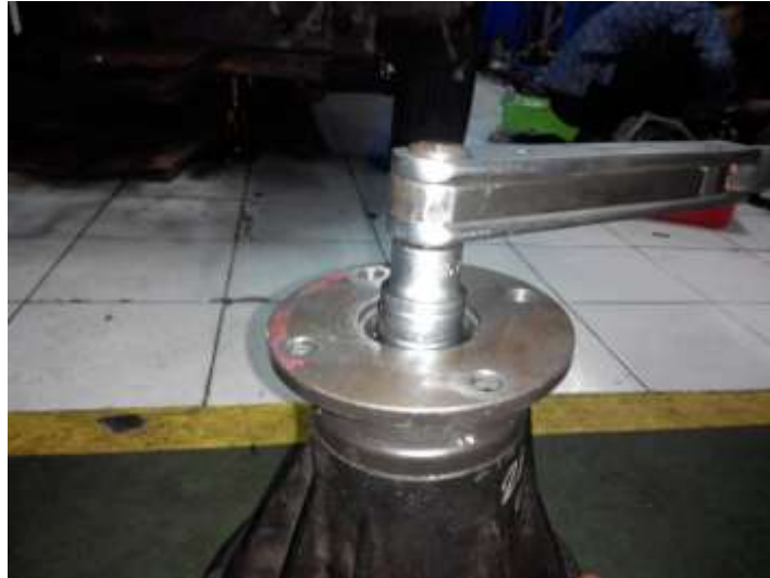
Gambar 3.15 Melepas Drive Pinion
