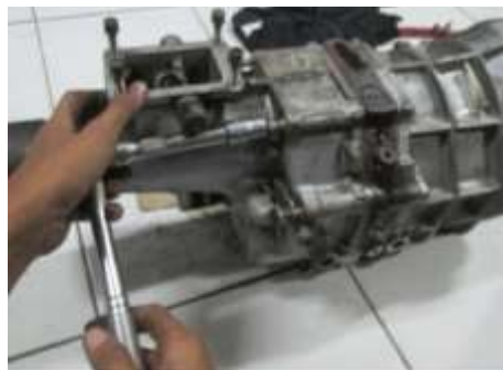
Gambar 3.7. Melepas baut extension housing
