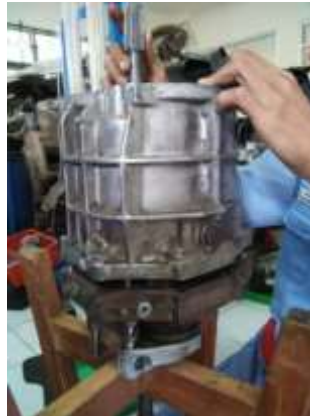
Gambar 3.8. Melepas transmission case
