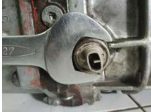
Gambar 3.41. Memasang speedometer driven gear
