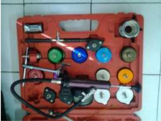
Gambar alat *radiator pressure tester*
