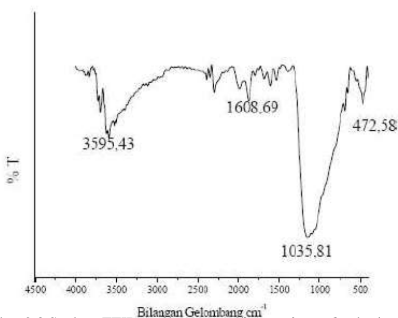
Gambar 2.3 Spektra FTIR ( Fourier Transform Infra Red ) abu layang PLTU Suralaya (Puspitasari, & Atmaja, 2010)
