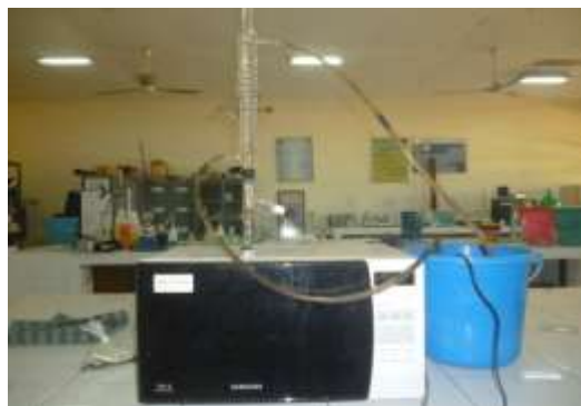
Gambar 5. Rangkaian Microwave Assisted Extraction
