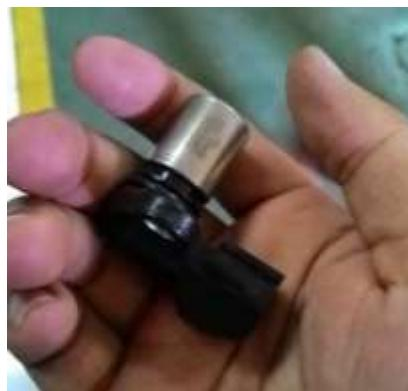
Gambar Memeriksa Kondisi *Camshaft Position sensor*
