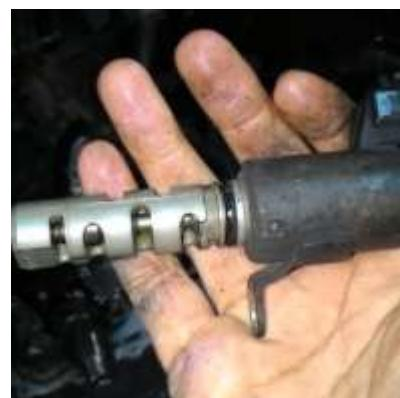
Gambar Memeriksa Kondisi *Camshaft Timing Oil Control Valve*
