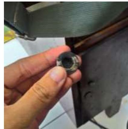
Gambar Tutup Stopper Plate Chain Tensioner
