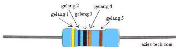
Gambar 2.7 Lima Gelang Warna Resistor
