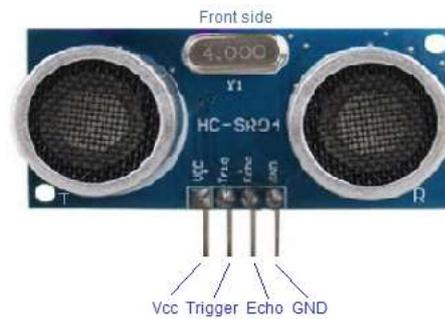
**Gambar 2.4** Sensor Ultrasonik HC-SR04 Tampak Depan
