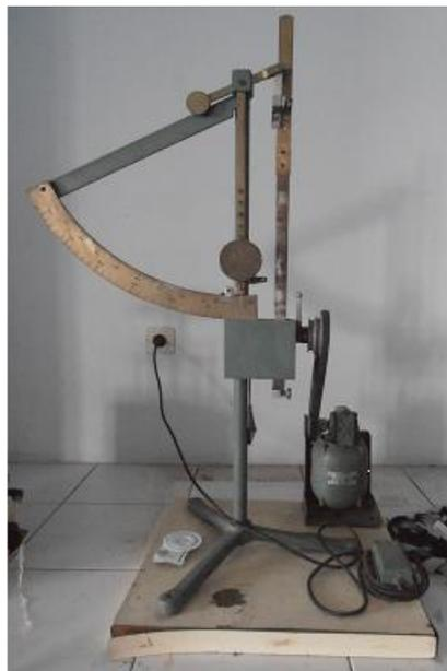
Gambar 3.2 Pendulum *tester* (sumber: data penelitian, 2013).
