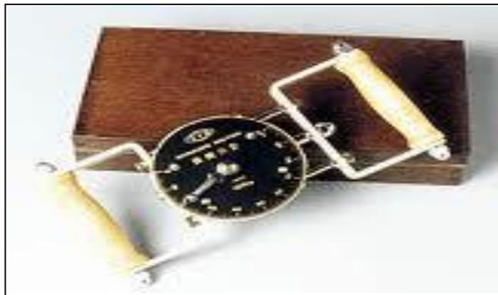
Gambar 3.2 *Pull and Push dynamometer*
