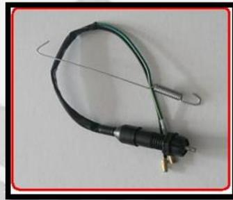
Gambar 3.18 Switch lampu rem belakang Yamaha Vixion
