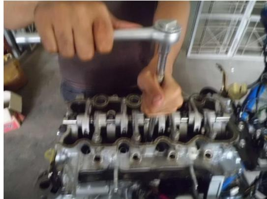
Gambar 55. Melepas *bolt cylinder head*.
