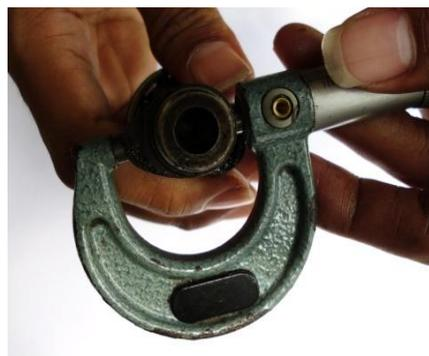
Gambar 57. Mengukur diameter panjang *camshaft*.
