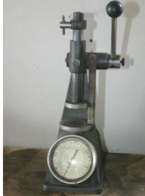
Gambar 38. *Valve spring tester.*
