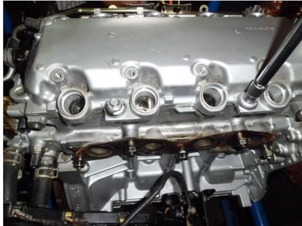
Gambar 47. Melepas baut *cylinder head cover*.
