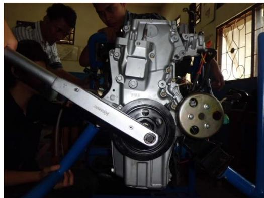
Gambar 48. Memutar *crankshaft pulley*.
