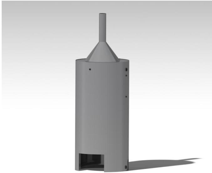
Gambar 4.7. *Vertical firetube boiler*
