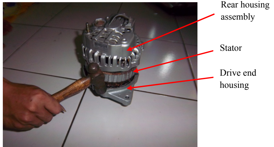
Gambar 3.5 Melepas drive end housing
