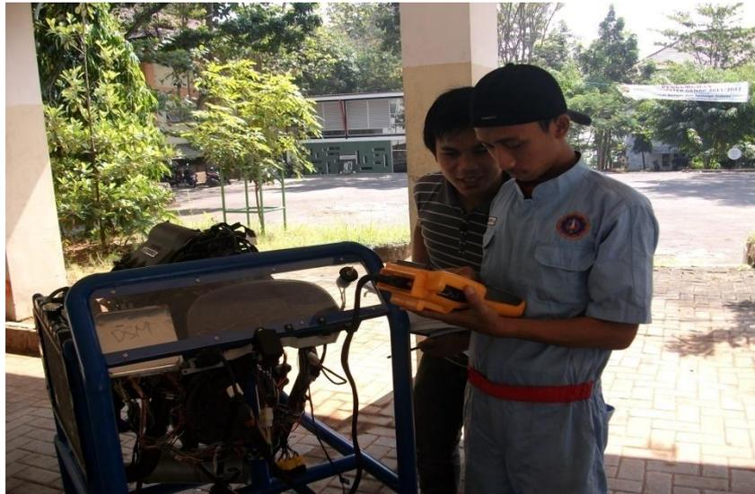
Gambar 3. Foto Pemeriksaan Menggunakan *Scanner*
