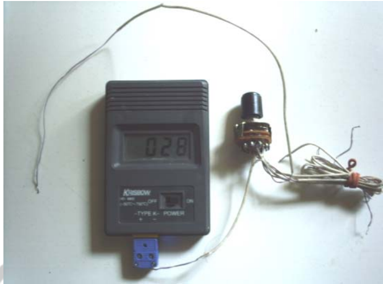
Gambar 05. Termokopel (Pengukur temperature bahan bakar)
