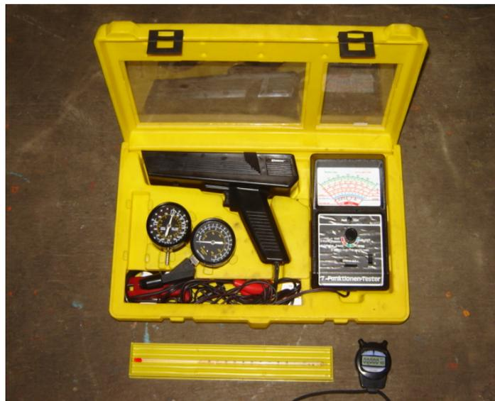
Gambar 30. *Timing lights, compression tester, tachometer, thermometer, stop watch.*
