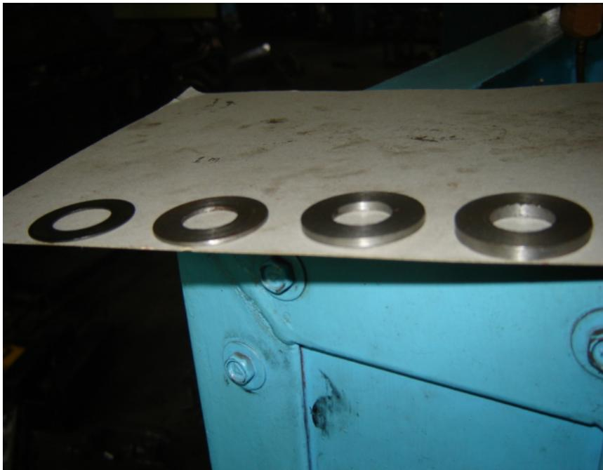
Gambar 28. shim pegas katup standar (0,5 mm), 1 mm, 2 mm, 3 mm.
