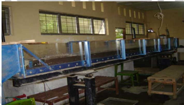
Gambar 10. Alat Recirculating Sediment Flume
